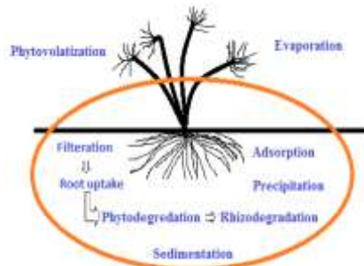
Fig 1: Mechanisms of construction wetland.
